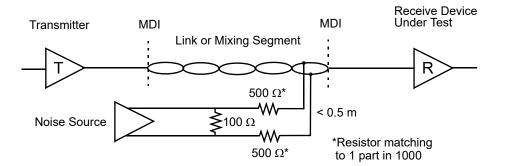
Figure 168–19—Alien crosstalk noise rejection test set-up
