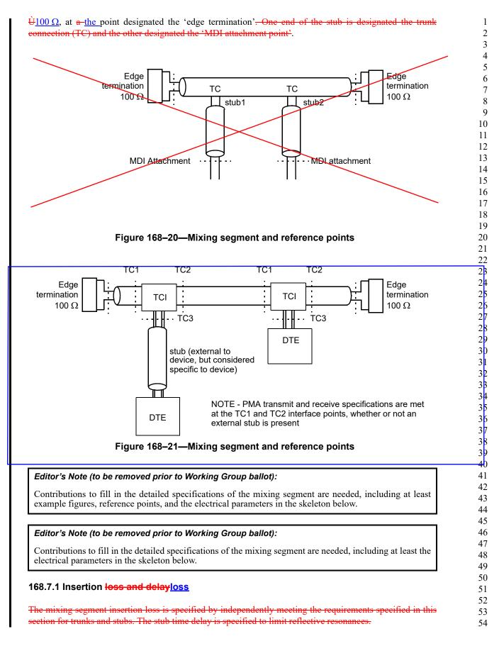
The mixing segment insertion loss is specified including any through-path insertion loss for the TCIs. See 168.8.2 for specification of the insertion loss and return loss (reflections) at the TCI interfaces.
